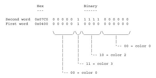
*Pointer Color Ordering.* The first word in a line gives the least significant bit of the color register and the second word gives the most significant bit.
