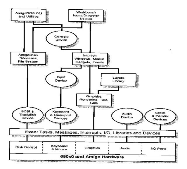
Figure 1-1: Amiga System Software Hierarchy
