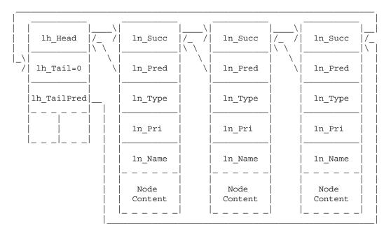
Figure 23-4: Complete Sample List Showing all Interconnections
