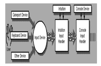
Figure 31-1: The Amiga Input Stream
