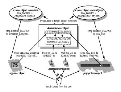
In this diagram, the application uses buttongclass Boopsi gadgets to send the rkmmodelclass the RKMMOD\_Up and RKMMOD\_Down attribute pulses.
