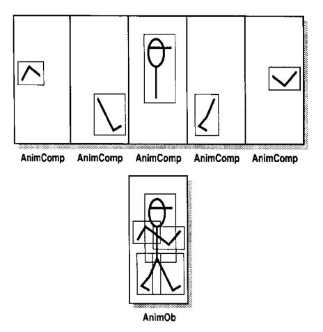
Figure 28-4: Linking AnimComps For a Multiple Component AnimOb
