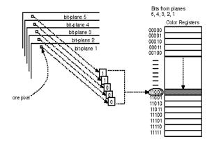
Figure 27-8: Bits from Each Bitplane Select Pixel Color
