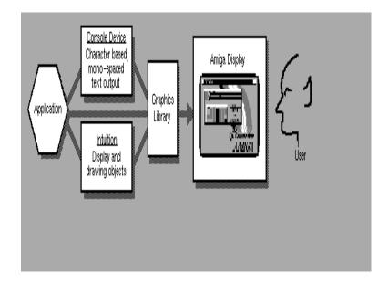
An application's display output can go through the high level interfaces of the console device or through the Intuition library. Additionally, display output may be sent directly to the graphics library. Notice that both the Console and Intuition call the graphics library to render to the display.
