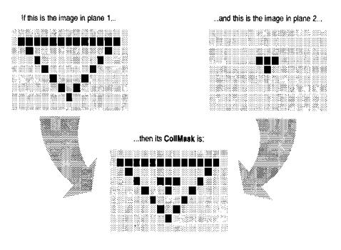
Figure 28-3: A Collision Mask
