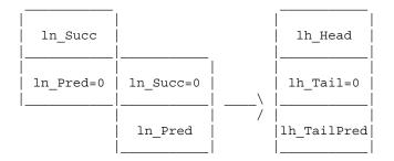
The **Ih\_Head** and **Ih\_Tail** fields of the list header act like the **In\_Succ** and **Ih\_Pred** fields of a node. The **Ih\_Tail** field is set permanently to NULL, indicating that the head node is indeed the first on the list -- that is, it has no predecessors. See the figure above.
